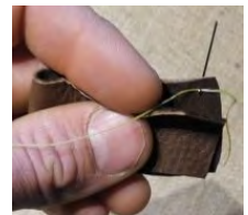
Illustration 8: First stitch: "Hiding the Knot"
