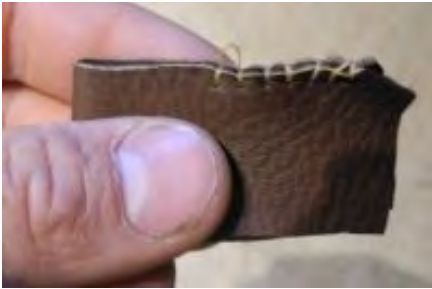
Illustration 9: Appropriate stitch length and stitch depth.
