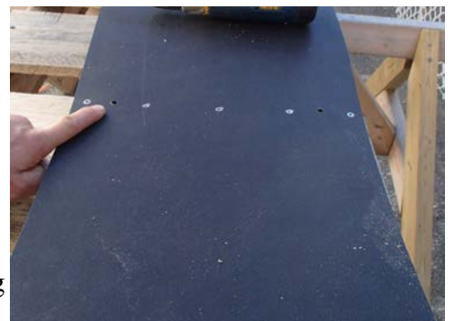
Illustration 9: Hole location in CB#2 for Haul Lines
