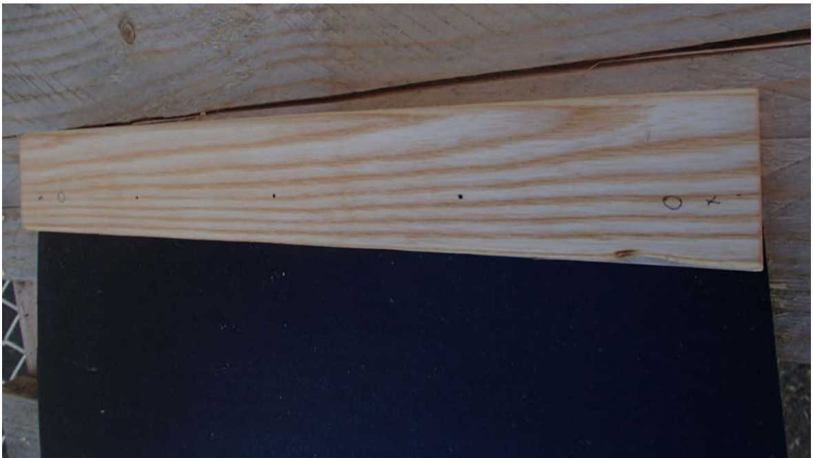
Illustration 10: Headboard layout showing location of screws and hole to accept running line.
