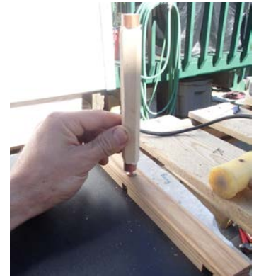
Illustration 15: Driving the Rivet Washer
