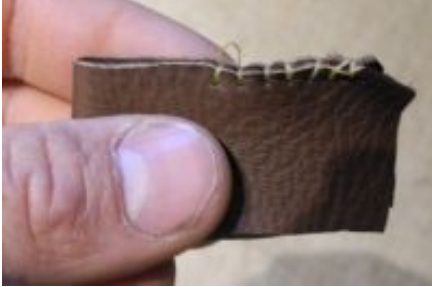
Illustration 11: Appropriate stitch length and stitch depth.
