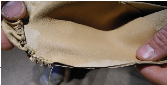
Illustration 14: Once the vamp and sole line up as shown, you are finished puckering!
