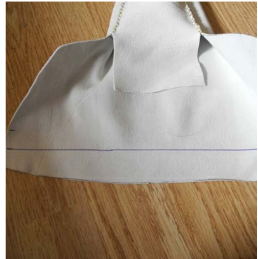
Illustration 18: Draw a straight line across the rear of your moccasin from point to point and trim. REMEMBER: this should be HALF the overlap measured!
