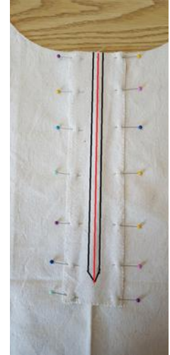
Illustration 15: Neck facing aligned on anorak front. Cut line in red, fold lines in black.
