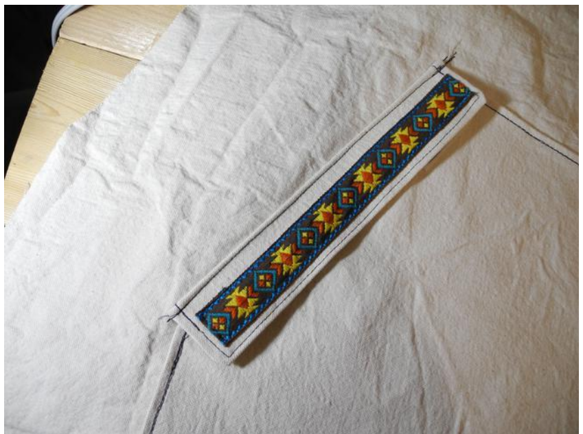
Illustration 19: Pocket flap AFTER top-stitching. Note how the stitching extends beyond the pocket flap slightly.
