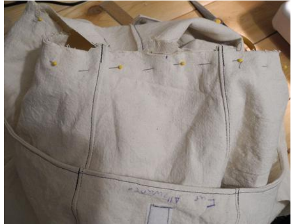
Illustration 30: Pinning the anorak hood to body. Note the short cotton "hangy loop" tails protruding past the seam.
