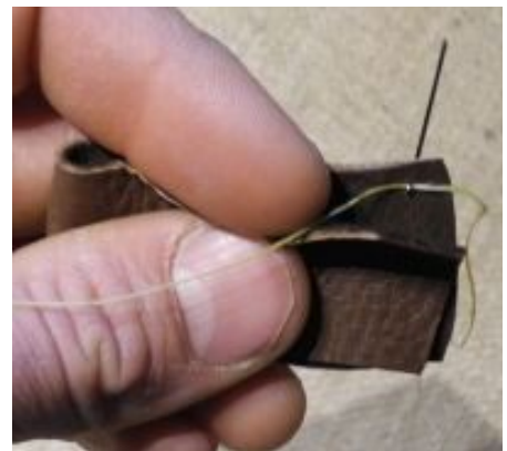
Illustration 8: First stitch: "Hiding the Knot"
