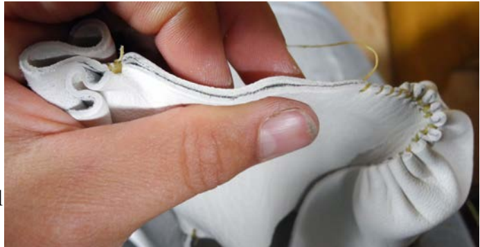
Illustration 12: Once the vamp and sole line up as shown, you are finished puckering!
