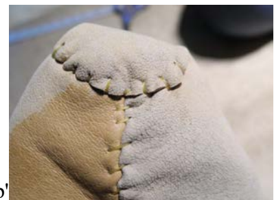
Illustration 19: The finished heel seam - showing a "closed" whip stitch.
