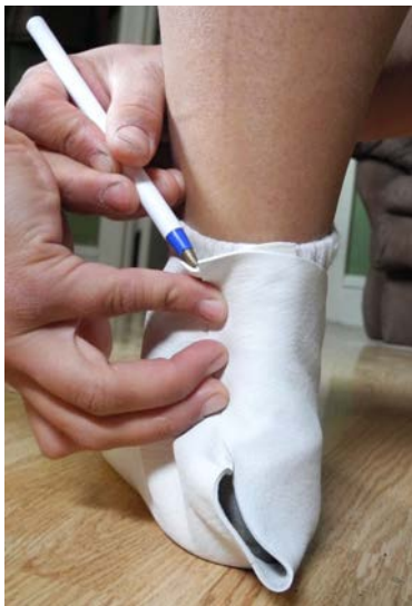
Illustration 14: Wrap the moccasin around your heel and mark the overlap.
